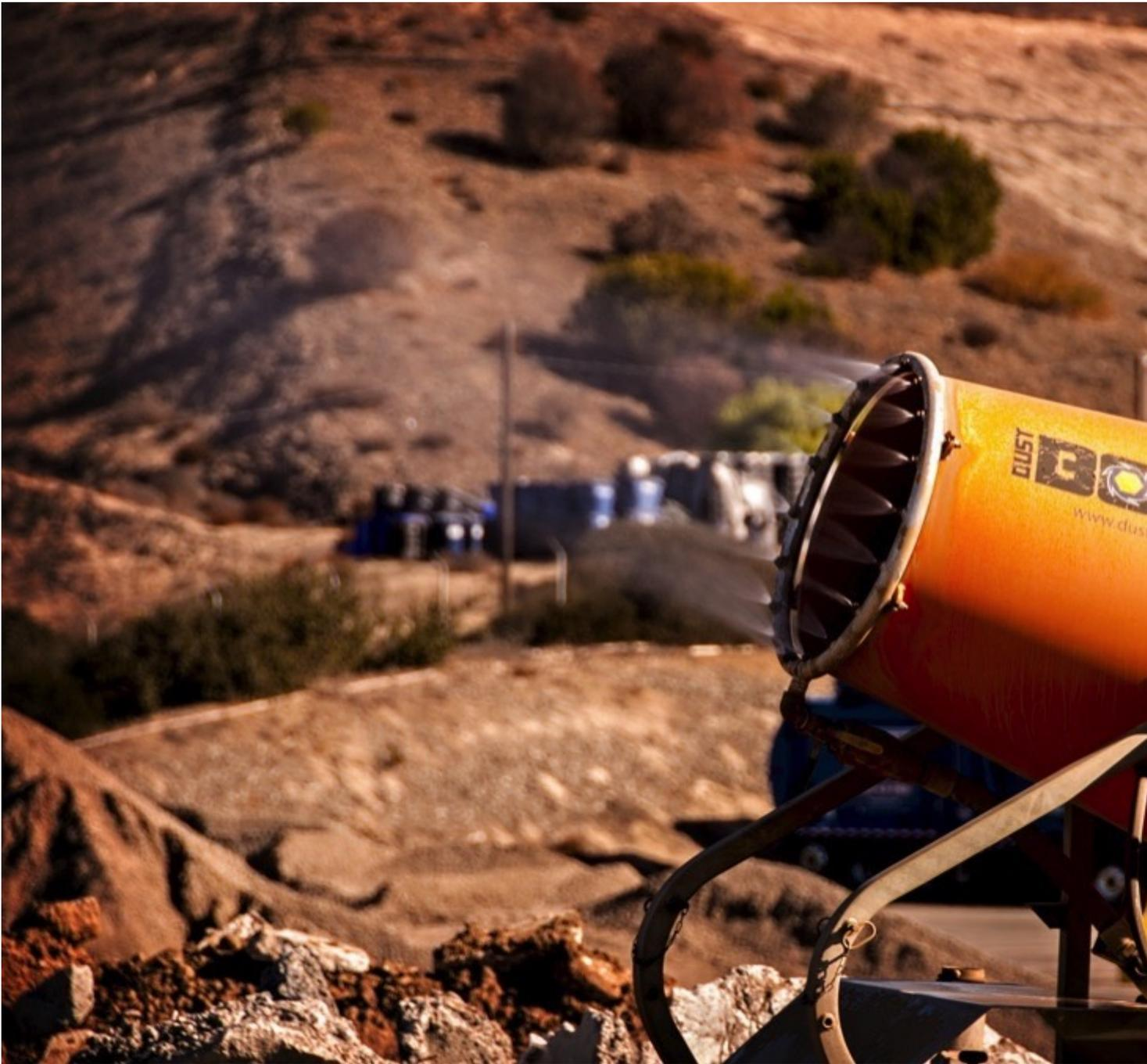
The Dustboss atomizer needs 11.3 GPM at 100 PSI to generate a dust catching mist.
