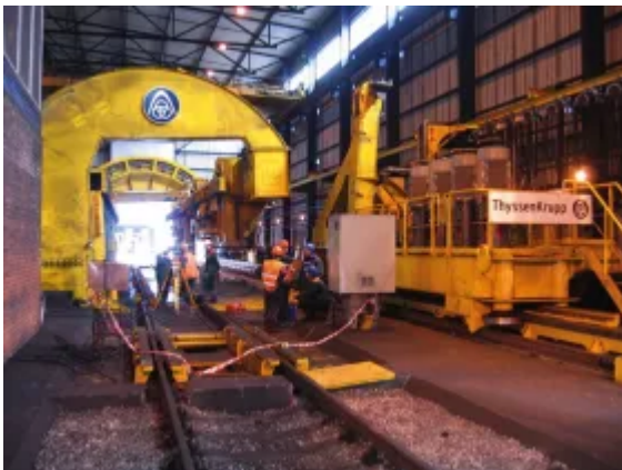
Fig. 4: Side arm charger with electro-mechanical drive and festoon arrangement for power supply.
