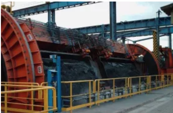
Fig. 2: Tandem tippler working at Vale's Tubarao Terminal, Brazil.
