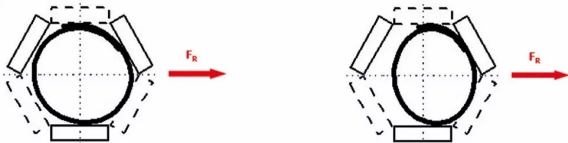
Fig. 8: Sufficient (left) and non-sufficient (right) transverse stiffness.
