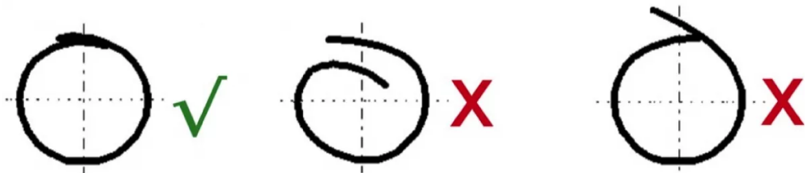
Fig. 7: Good (left) and unsuccessful designs of the tube belt (middle and right).
