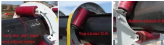
Fig. 14: Position of the belt overlap.
