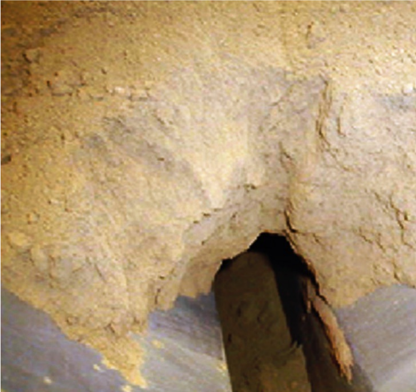
Fig. 5: An iron oxide powder arch in a Vee hopper.
