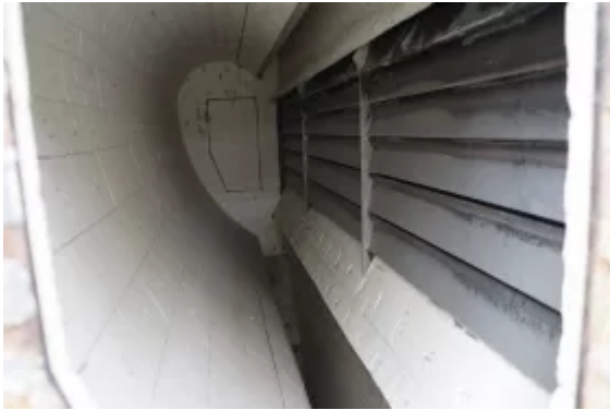
Fig. 4: Ceramic linings and vanes inside one of the G1 classifier units to the left; after 8 years of operation, the wear of the linings is still negligible. (Picture: © Metso Minerals)
