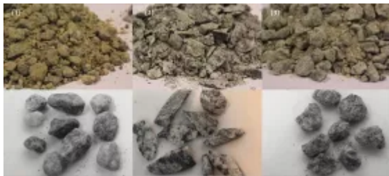
Fig. 2: Different types of fine aggregates: (1) High-quality, 0/8 mm natural glaciofluvial sand from Norway; (2) Low-quality, 0/8 mm co-generated material of coarse crushed aggregate production (should not be called crushed or manufactured sand); (3) High-quality, 0/8 mm crushed sand, produced using an optimized crushing circuit and VSI shaping. (Picture: © Rolands Cepuritis)
