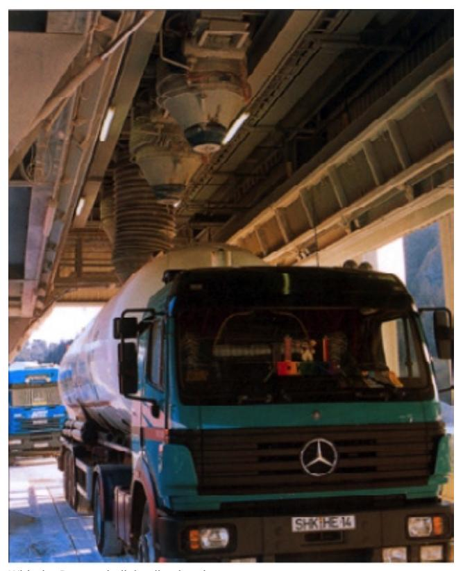
With the Beumer bulk loading head, bulk transporter vehicles can be loaded quickly and without dust.
