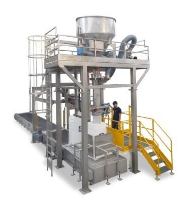
The new net weighing and filling station for single loop bulk bags can fill up to 180/BB per hour. (Picture: ©Concetti)
