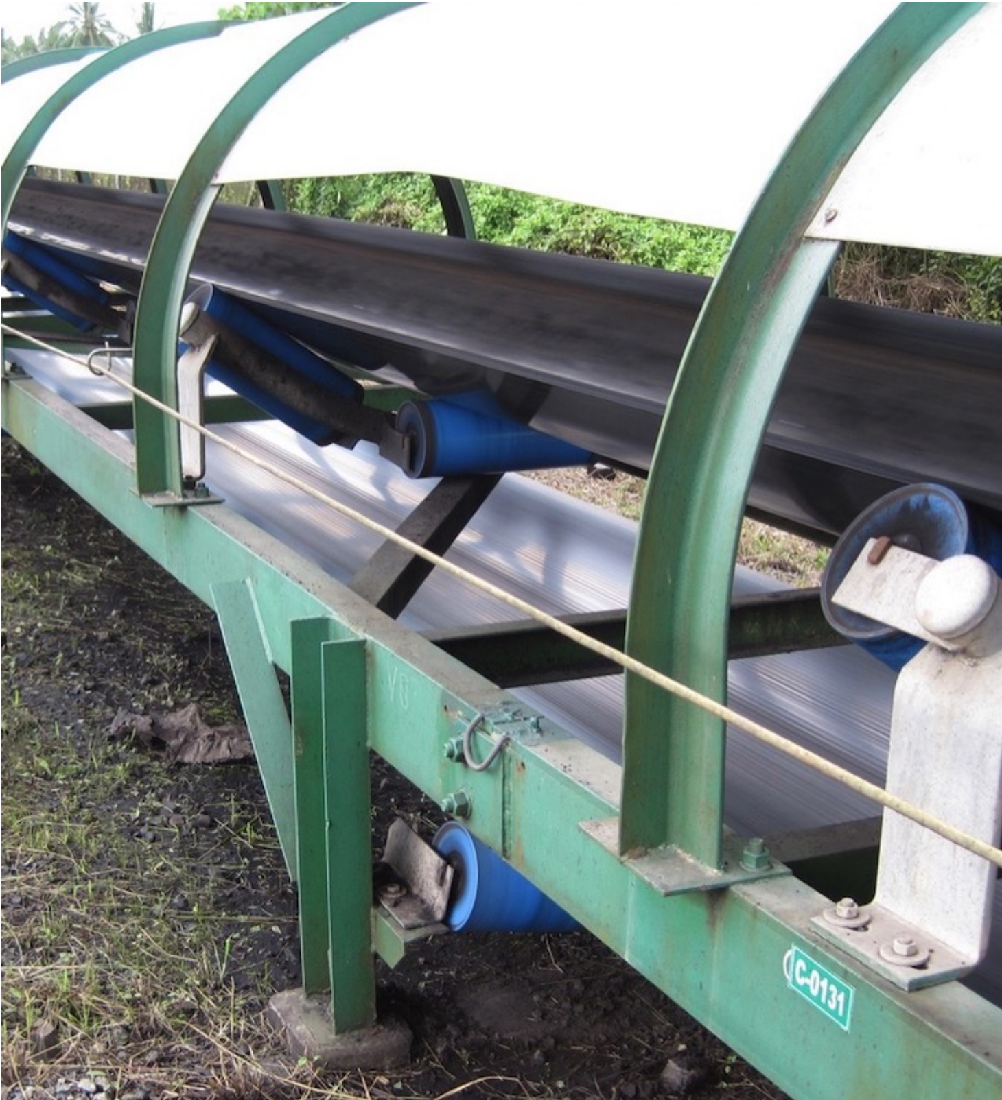
Fig. 1: Artur Küpper optimised idlers in action. (Pictures: Artur Küpper GmbH & Co. KG)
