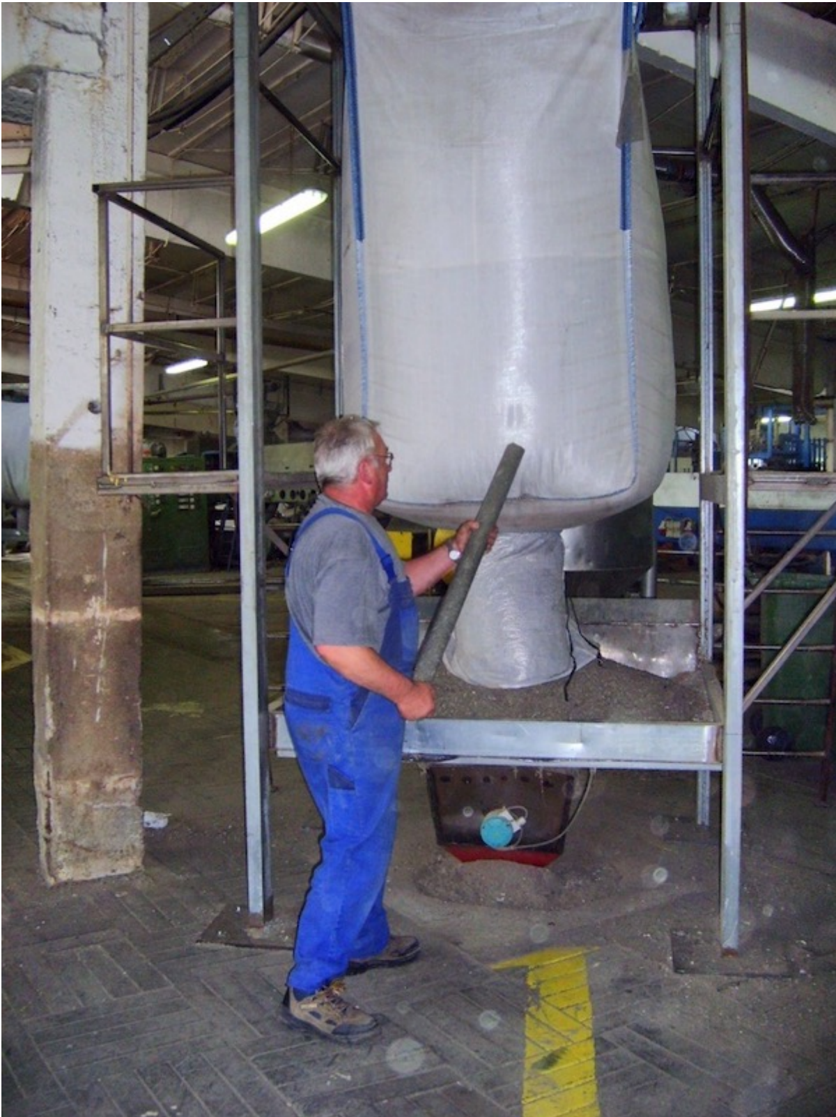
Fig. 1: New secondary raw materials, such as plastic grinds or flakes, pose new challenges for manufacturers due to their problematic flow behaviour (Pictures: Alfred Sonntag)
