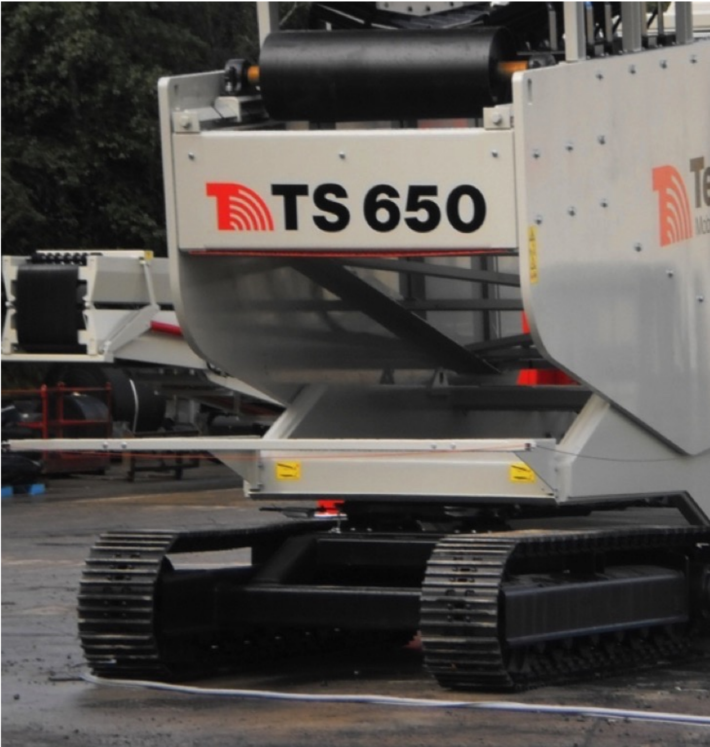
Fig. 2: A remote controlled tracked dolly unit ensures mobility on harsh ground conditions.
