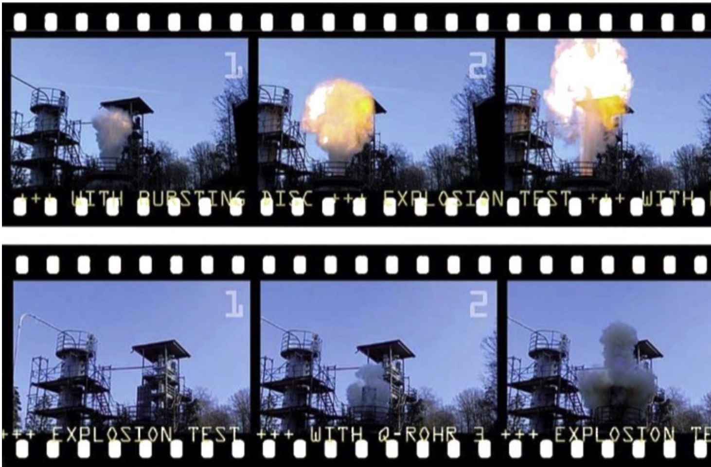
Fig. 1: Flameless venting systems not only extinguish the flame automatically, also the pressure rise and increased noise level associated with free vented explosions are massively reduced. (Pictures: © Rembe GmbH)
