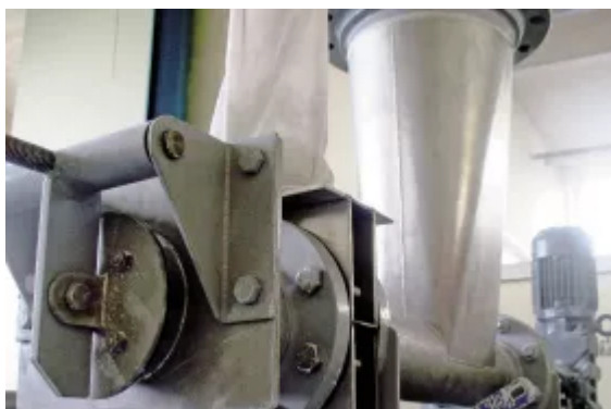
Fig. 1: Plug-screw feeder technology allows biomass energy companies to successfully overcome the challenge of both feeding pyrolysis and gasifier processes. (Pictures: © Ajax Equipment Ltd.)
