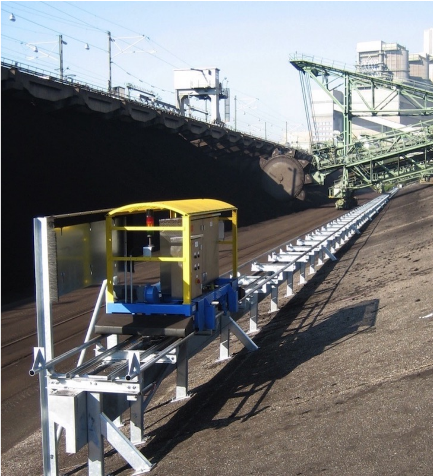
Fig. 1: 3D scanners deliver information for stockpile monitoring and visualisation in an integrated coal management system. (Pictures: © ABB)
