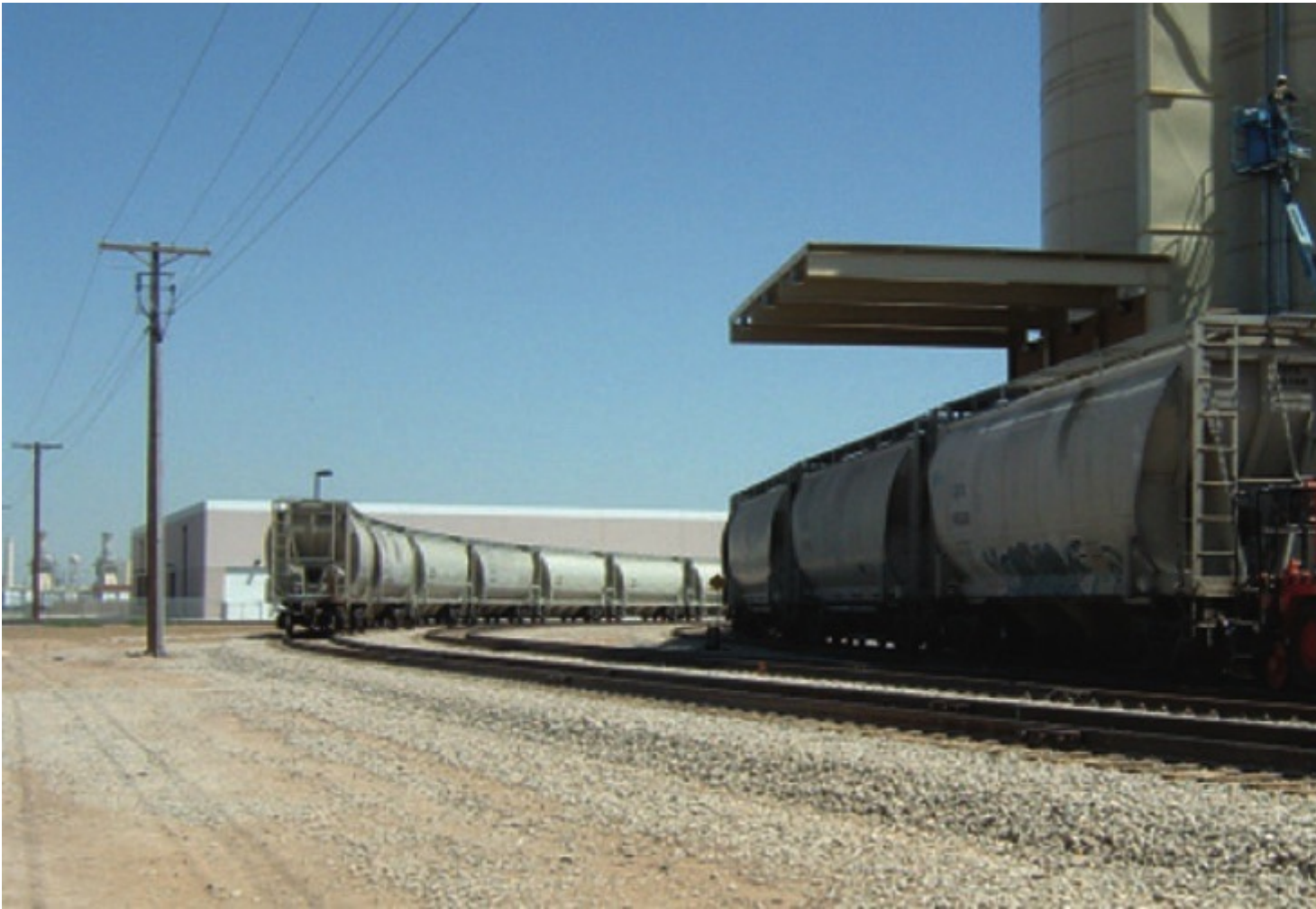
Fig. 9: Bulk cement railcars loaded at a silo.
