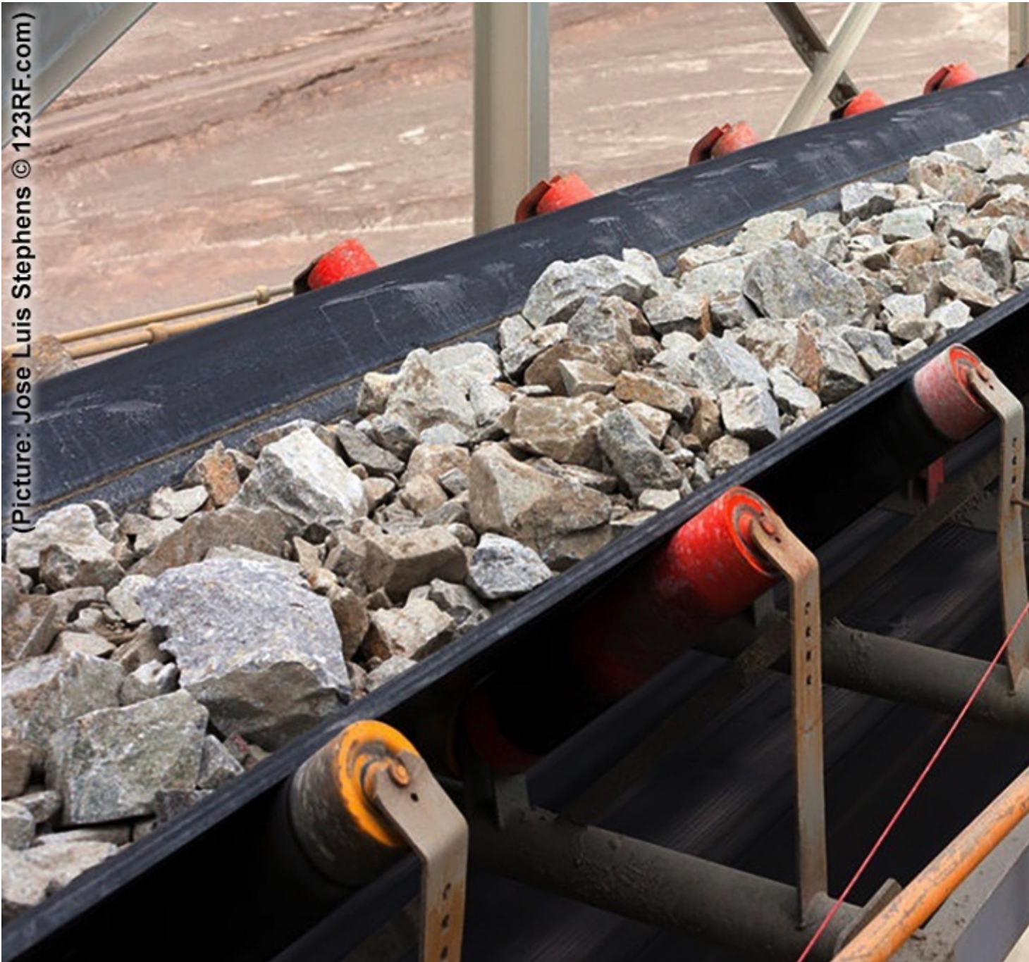
Fig. 1: Conveyor belt indentation can be the primary source of power loss in driving a long horizontal belt conveyor.
