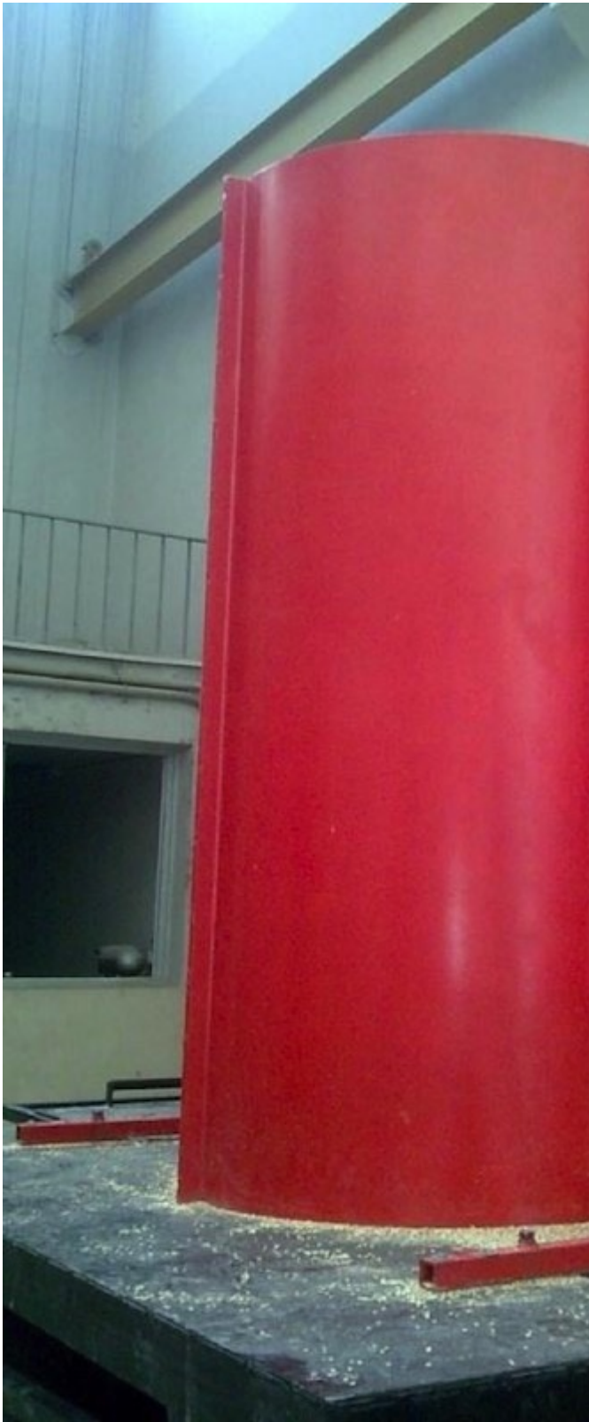
Fig. 2: Study model silo with mounting points of the pressure cells. (Pictures: University of Damacus)
