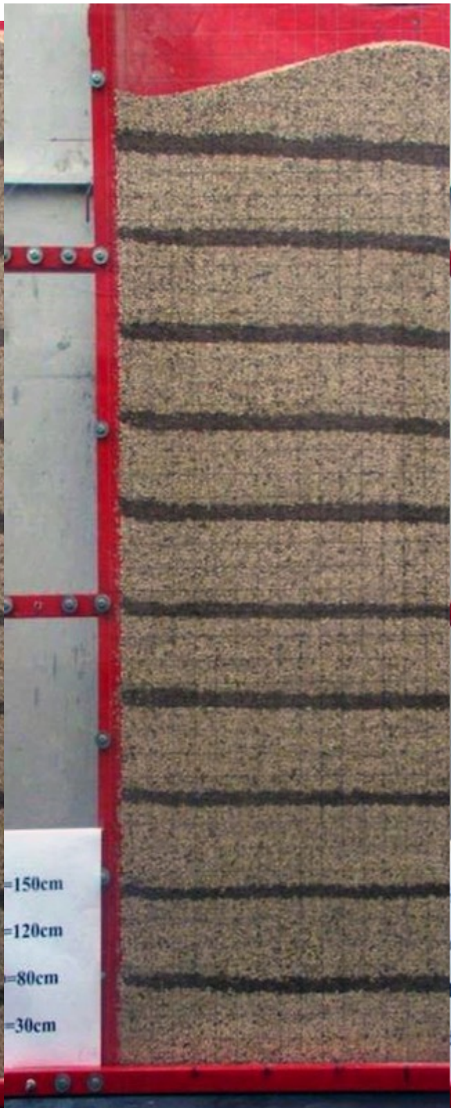
Fig. 6: Eccentric outlet discharge ( e/R = 0.5 ).
