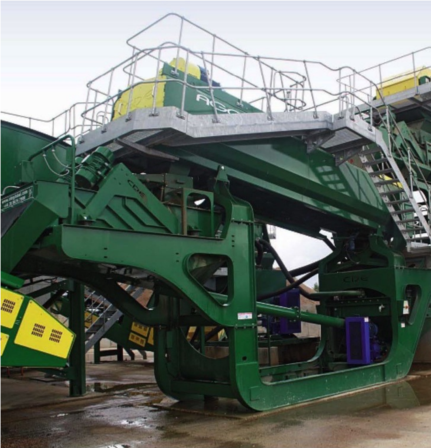
Fig. 3: The AggMax involves four stages of processing in one unit, pre-
