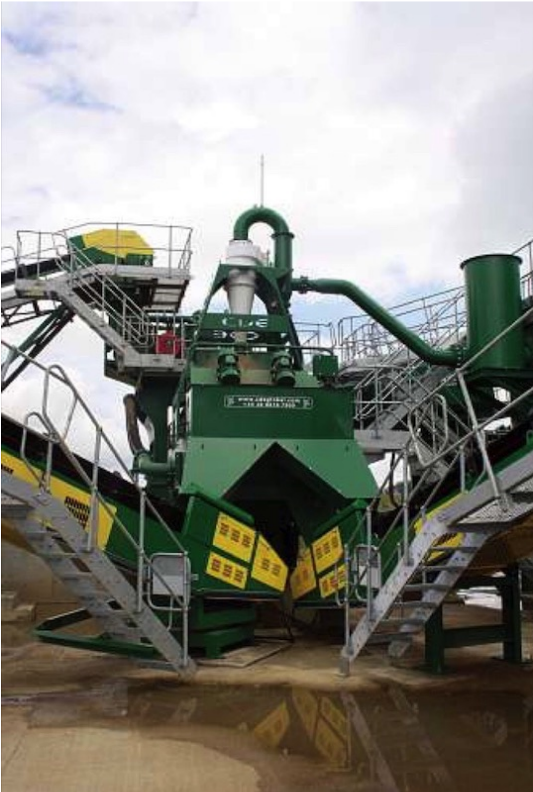
Fig. 4: The -5 millimetre material and waste water are sent to the Evowash sand washing plant to maximise recovery of the sand fraction.
