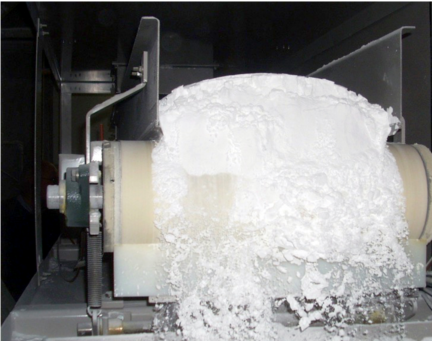
Fig. 3: The weighfeeder handles material flow ranging from 500 kilograms to 6 tonnes per hour.
