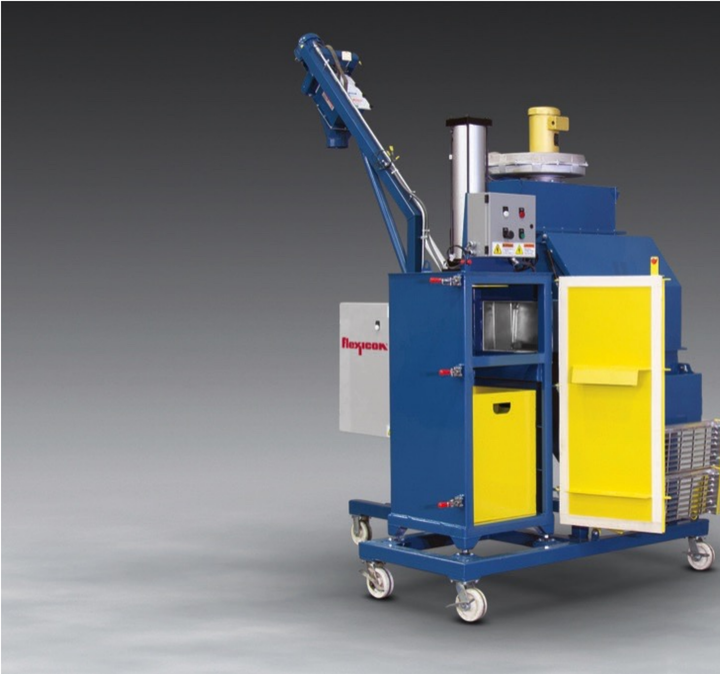
Fig. 2: Dust generated from bag dumping, pass-through of empty bags, and bag compaction, is drawn onto cartridge filters equipped with air nozzles that dislodge dust
