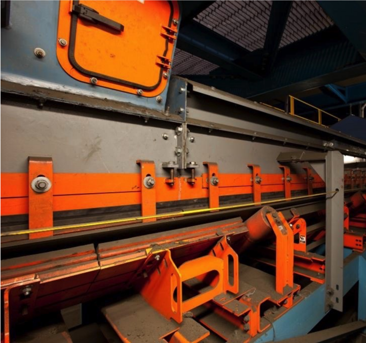
Fig. 3: Martin® ApronSeal Skirting is a dual-sealing system, with a primary seal clamped to the steel skirtboard and an “outrigger” strip to capture
