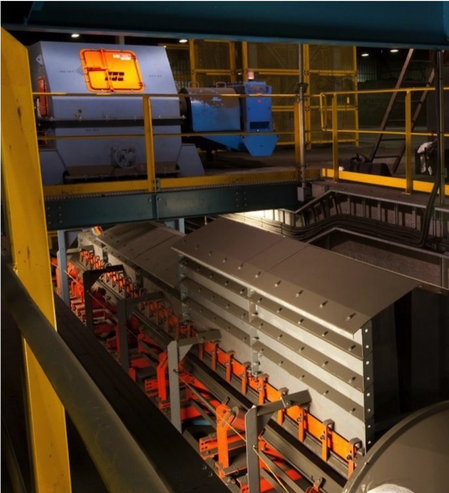
Fig. 2: The extended height settling zone from Martin Engineering is designed to decrease air velocity and increase settling time.
