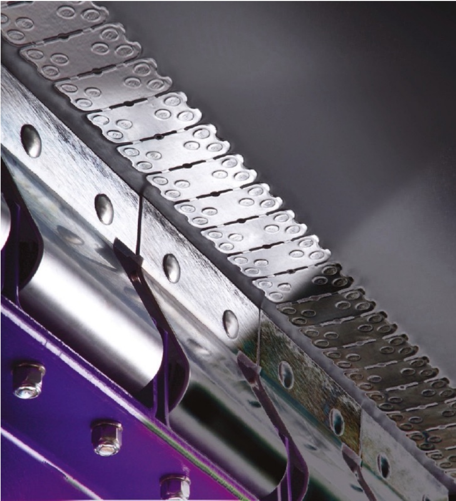
Fig. 2: If the fasteners and belt cleaners aren't compatible, the operator could have a serious problem.
