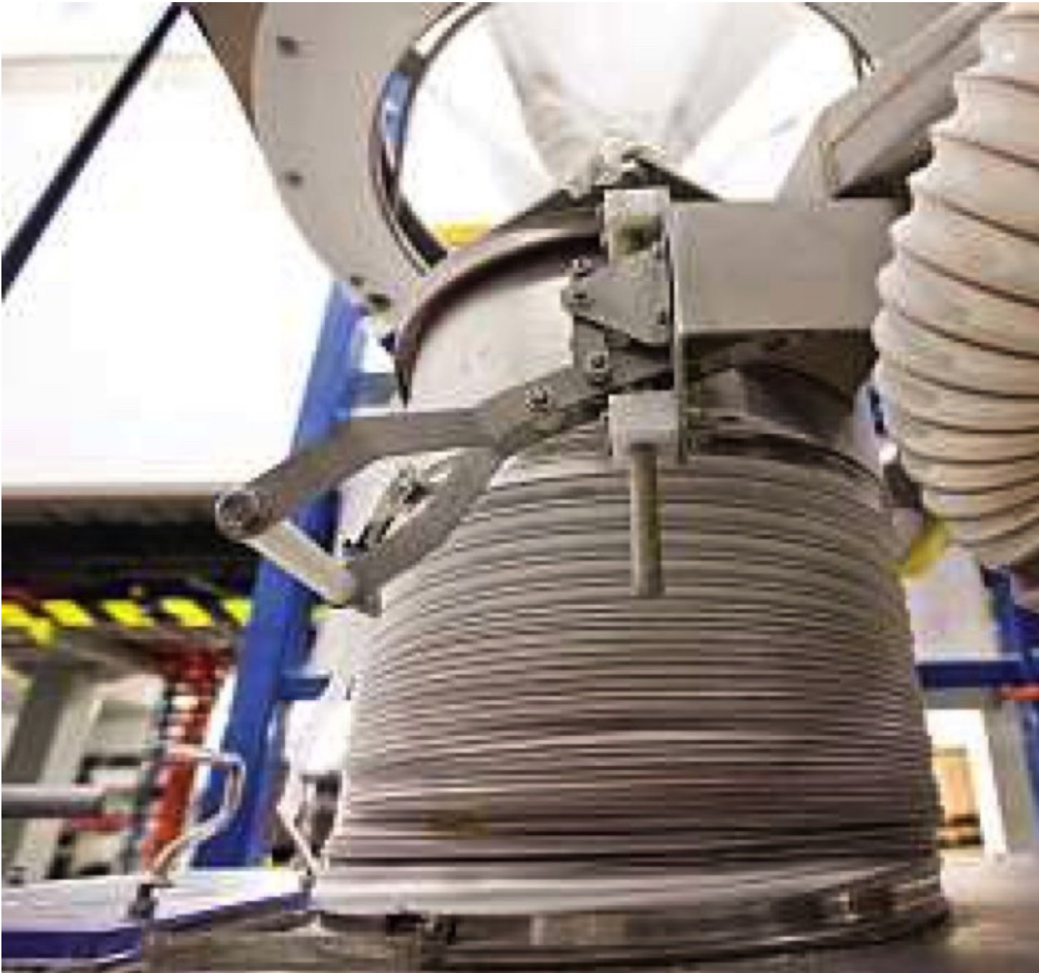
Fig. 2: Double wall Tele-Tube telescoping tube provides extra protection against dust leakage during transfer from the bag. Tube is secured to the bag spout by a Spout-Lock clamp ring that creates a dust-tight seal.
