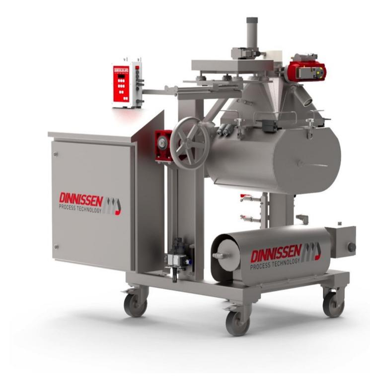
For this project, Dinnissen's engineers developed a very compact Pegasus® R&D mixer in which all raw materials can be kept in motion for long periods of time
