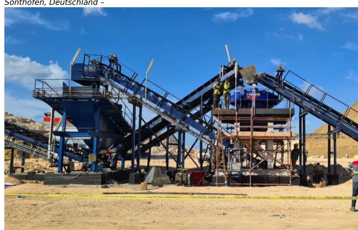
Cement manufacturer Amreyah Cement relies on crushing technology from BHS-Sonthofen to produce slag sand in its plant in Egypt.
