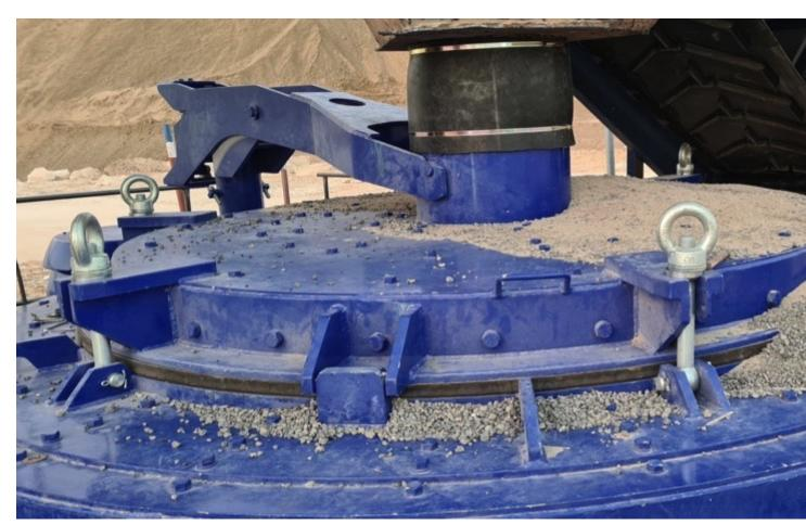
The BHS rotor centrifugal crusher of type RSMX 1222 is equipped with an anvil ring to produce fine-grained slag sand.
