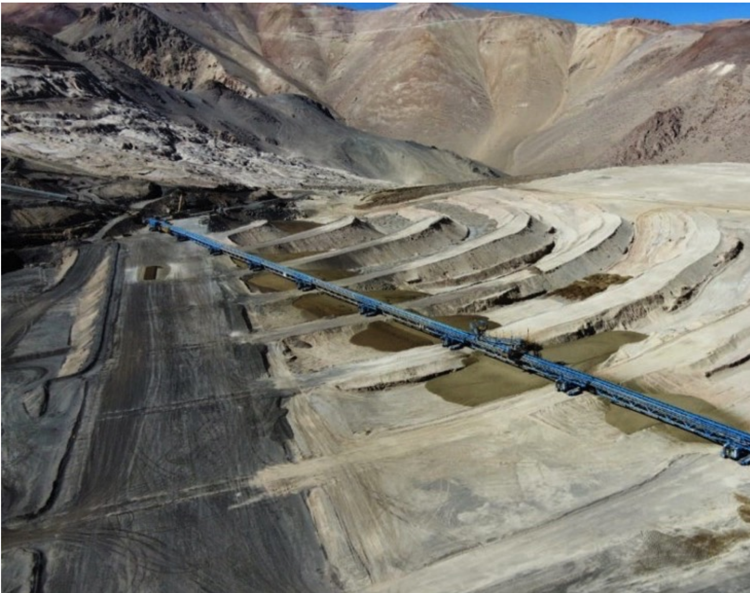
BEUMER Minerals & Mining Mobile Conveyor Bridge on Crawlers MSB1000.9. (Picture: ©BEUMER Minerals & Mining)
