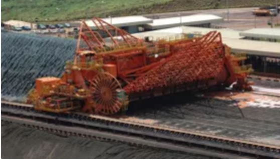
Fig. 1: The best homogenising efficiency is achieved while reclaiming at once from the full face of a stockpile, e. g. with a drum reclaimer. (Pictures: TAKRAF GmbH)
