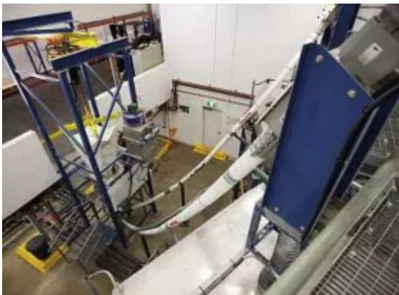
Fig. 3: Powder remains enclosed from the time it is received until it enters the mixing tanks.
