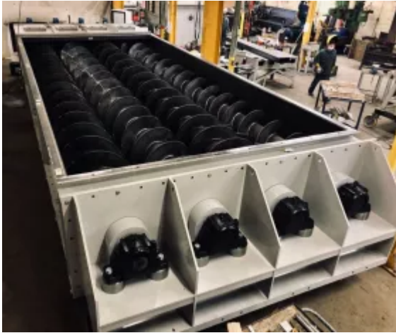
Quadruple Screw Feeder designed to work with poorly flowing refuse to provide a regular feed.
