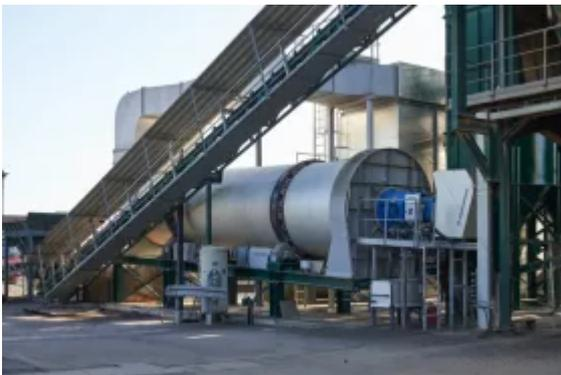
At the heart of the asphalt mixing plant in Aichach is the EVO JET 3 multi-fuel burner from Benninghoven.
