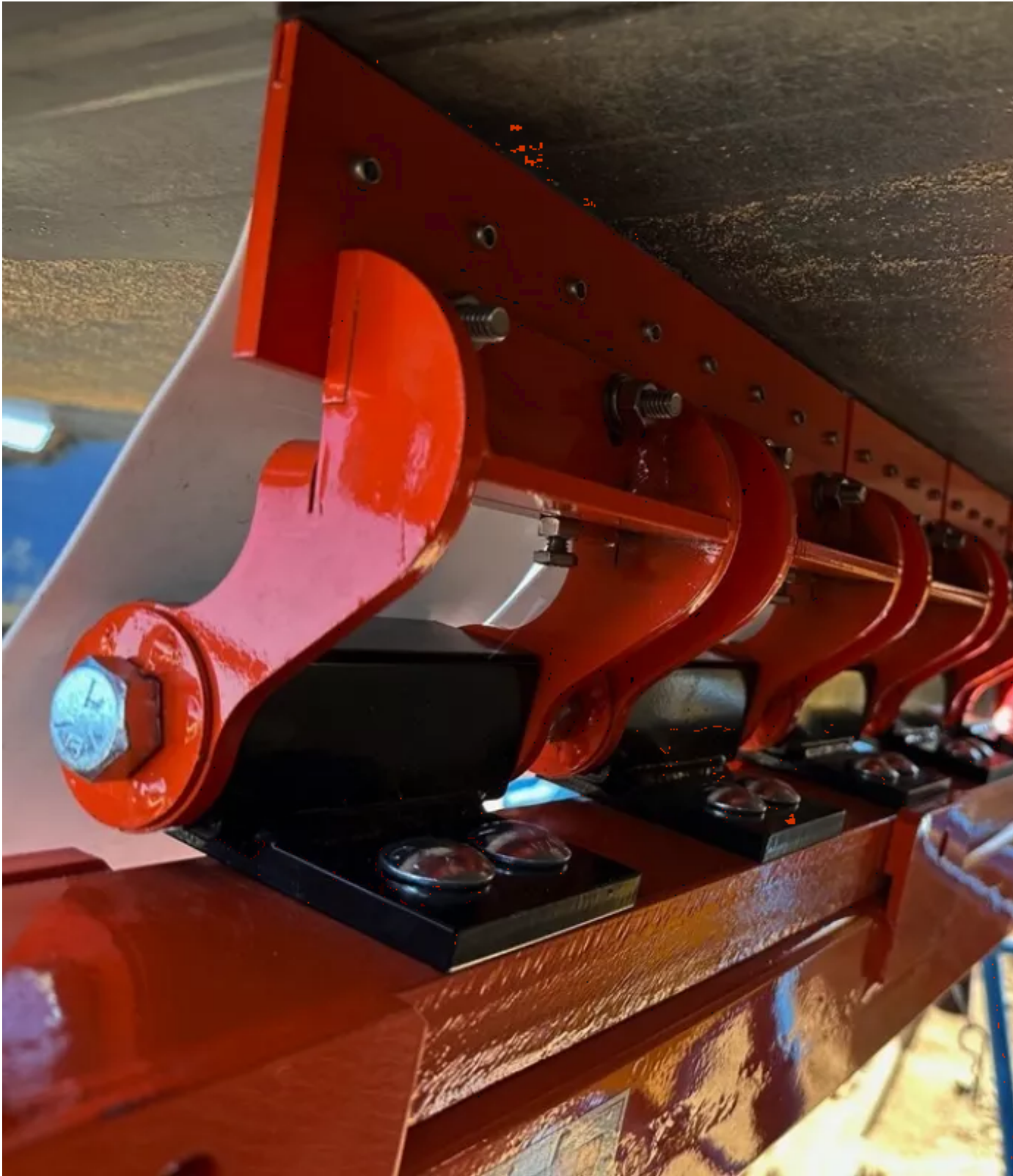
Cartridges with individual tensioning improves cleaning efficiency and effectiveness.
