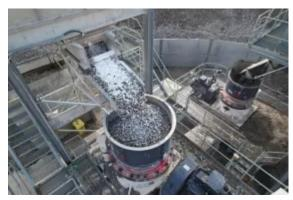
The setup included two Terex MPS MC320 cone modules and two Terex MPS MHS6203 screen modules.
