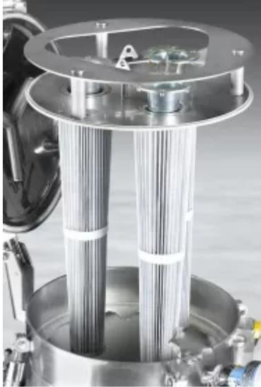
Hinged lid allows rapid removal of tapered filter cartridges, and unobstructed interior access for sanitising and visual inspection of material contact surfaces.
