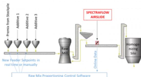
SpectraFlow Airslide Analyzer in the Puttalam clinker production process. (Pictures: ©SpectraFlow Analytics AG)
