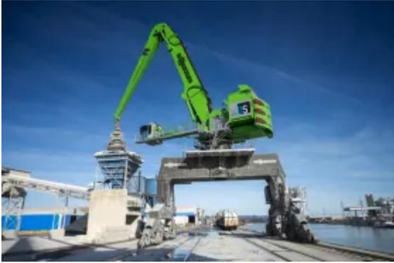
The world's largest 895 E Hybrid port material handler with 420 t operating weight. Here in the version with rail gantry in Austria.
