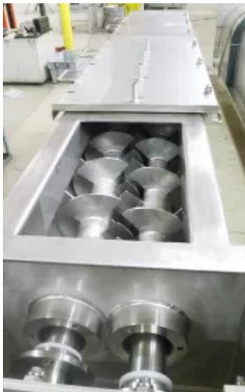
All four of the mixers include spray bars allowing water to be added to the dry salt; the mixers also each feature hinged stainless steel covers enabling the machines to be easily inspected.
