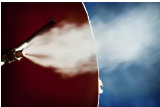
The Odor X Atomizer nozzle creates droplets as small as 15 microns to distribute the deodorizing chemical.
