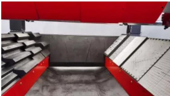
As alternatives to steel, rubber, ceramics and composite systems made of these two materials are generally considered for wear protection in conveyor systems.
