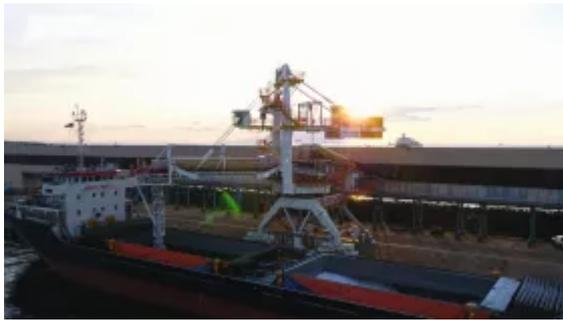
In the port environment, ship loaders ensure the fast, reliable loading of ships with bulk materials – for example urea fertilizers.
