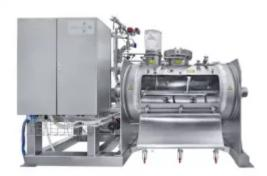
As the example of chewable tablets for dogs and cats shows, Ploughshare® Mixers can meet the specific requirements particularly well in several respects. (Source: Lödige Maschinenbau)
