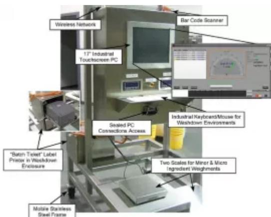
Semi-Automatic Hand Prompt Batching System (Picture: Sterling Systems & Controls)
