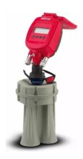
The 3D level sensor measures and maps multiple points on the material surface. Measuring irregular material surfaces ensures improved accuracy when calculating volume. Its accompanying 3DVision software shows a 3D image representing the topography inside the silo. This image indicates buildup that can cause sidewall damage in the silo and cone up or down conditions. MultiVision software allows viewing of multiple silos at a single location.
