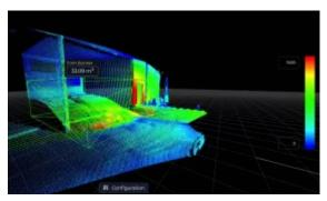
The solution provides 3D representations of bulk material piles. When the new Smart LiDAR Qb2 by Blickfeld is used, there is also the option to output only the volume value, significantly reducing the amount of data to be transmitted. (Copyright: Blickfeld)
